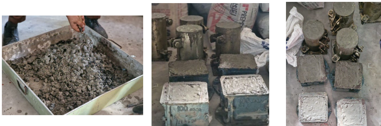
Figure 2: Casting, Molding, and Curing
