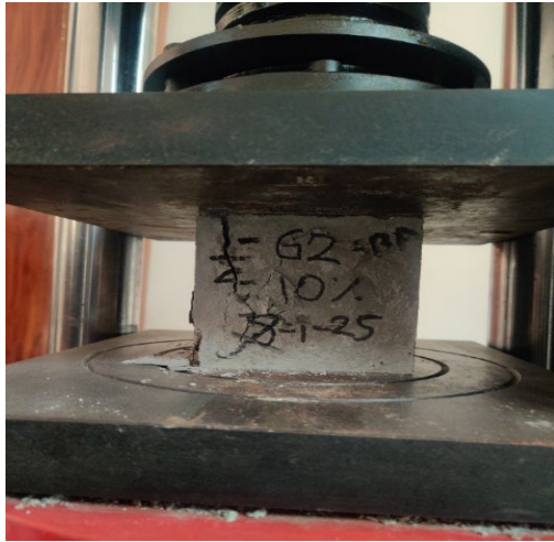
Figure 2: Compressive Strength Test
