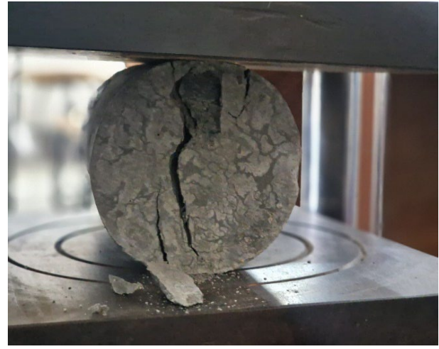
Figure 3: Tensile Strength Test
