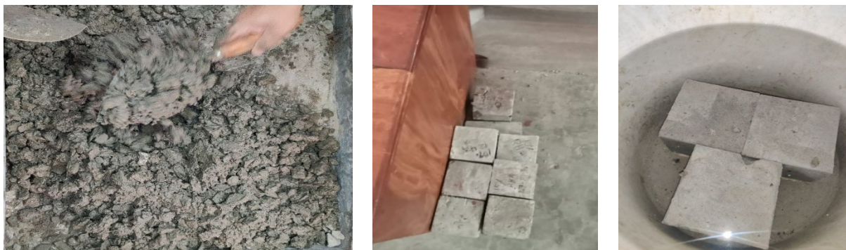
Figure 1: Preparation, Casting, and Curing of Specimens
